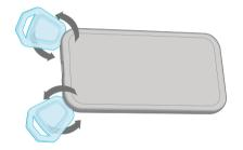
SLAM ships fully assembled. To open, use the included case key to separate the case.
